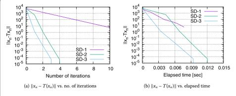
Figure 2 Evaluation of  $||x_n - T(x_n)||$  in terms of the number of iterations and elapsed time for Algorithms SD-1, SD-2, and SD-3 for Problem 3.1 when  $d := 10^4$ .
